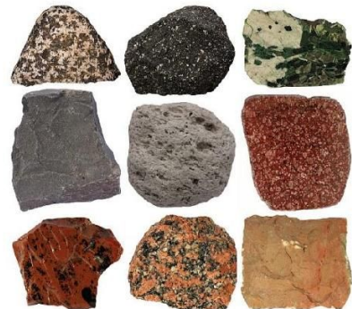
Igneous rocks from left to right: gabbro, andesite, pegmatite, basalt, pumice, porphyry, obsidian, granite, and tuff
