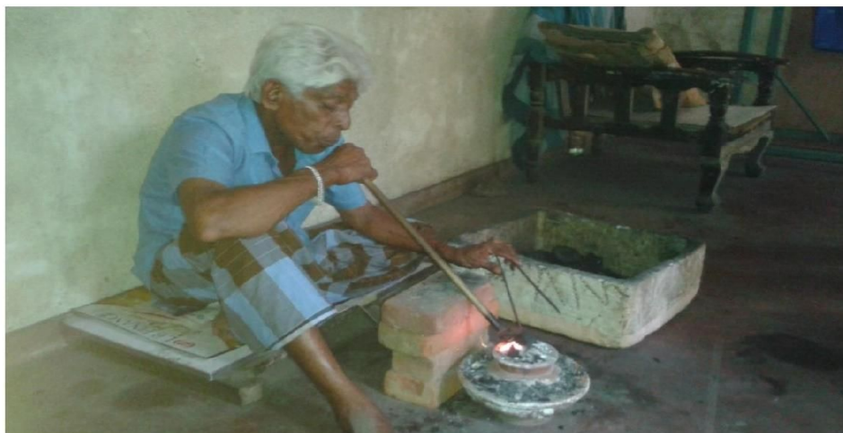
Figure 01: Operation of Blow pipe with one person (Location: Demmuwatta, Ratnapura, Sri Lanka)
