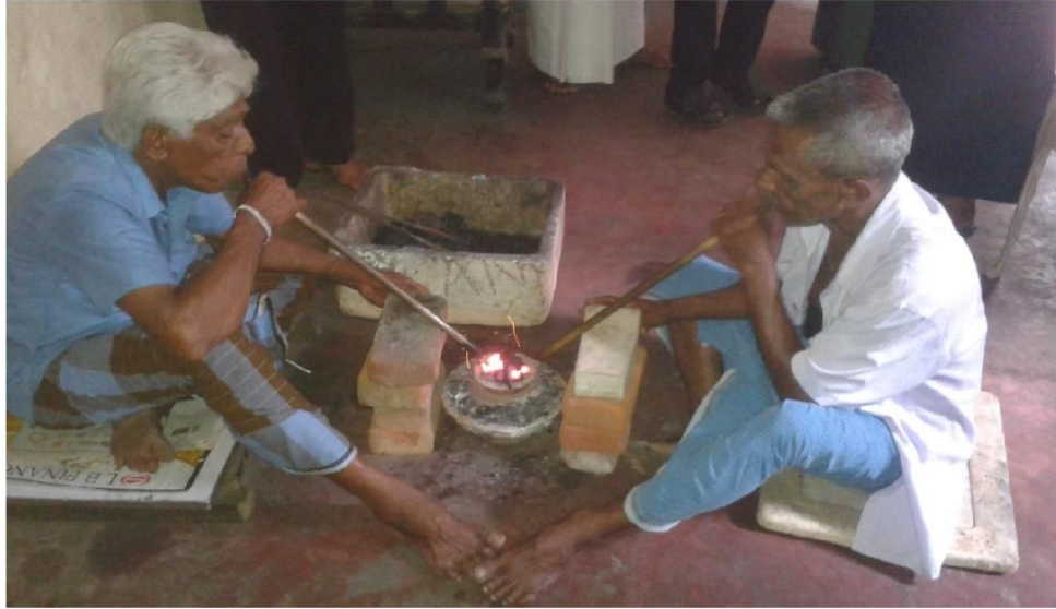
Figure 02: Operation of Blow Pipe with two people (Location: Demmuwatta, Ratnapura, Sri Lanka)
