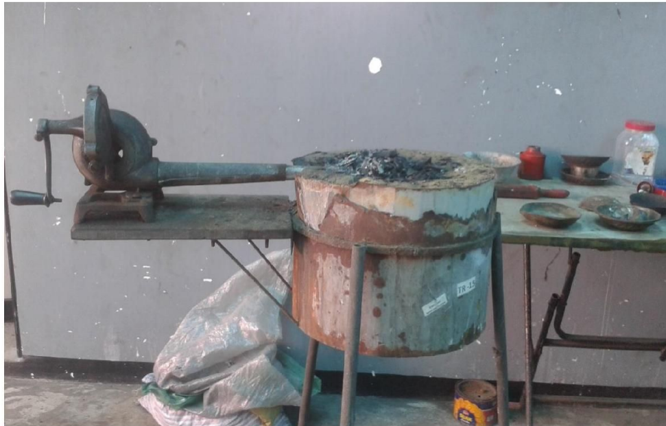
Figure 03: Mechanical Blow Pipe (Location: Demmuwatta, Ratnapura, Sri Lanka)
